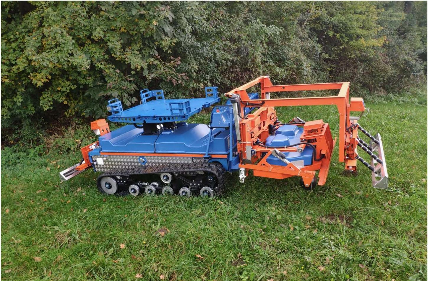
*Whenever needed, the Slopehelper can be operated by full manual remote control* Slopehelper
