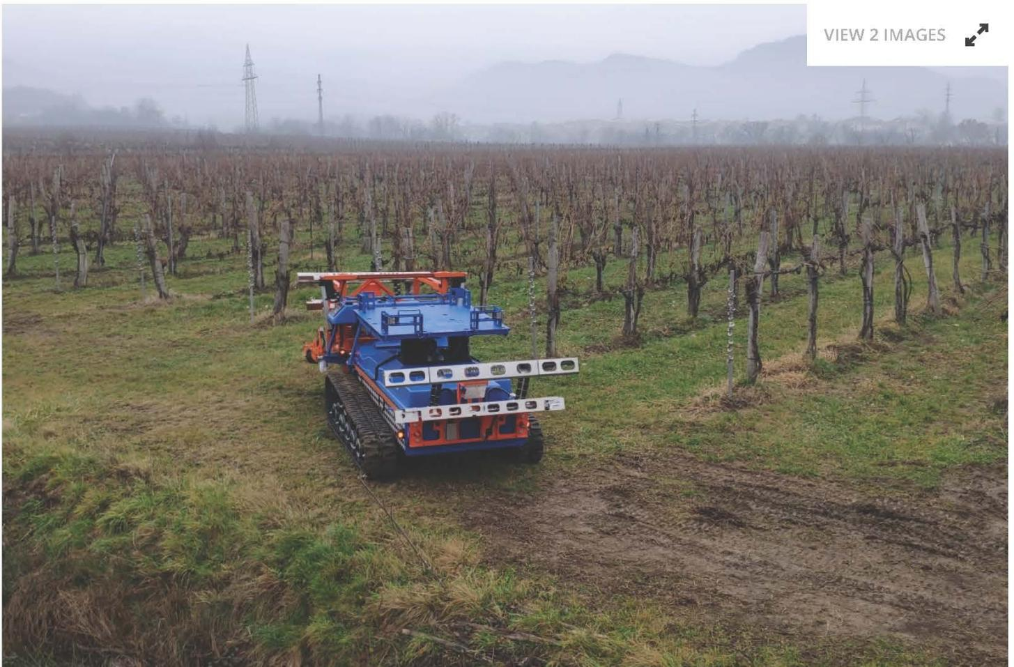
*The Slopehelper weighs a claimed 1,200 kg (2,646 lb) and is 2.6 m long (8.5 ft)* Slopehelper
