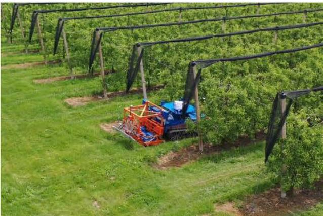
Slopehelper can carry tanks, bins/containers (for harvested products), people (for inspection, sorting) and machines and implements. - Photo: Slopehelper
